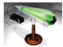
The Experiment An obstacle was placed between the cathode and the wall of the tube. A shadow of the obstacle appeared at the end of the tube.
